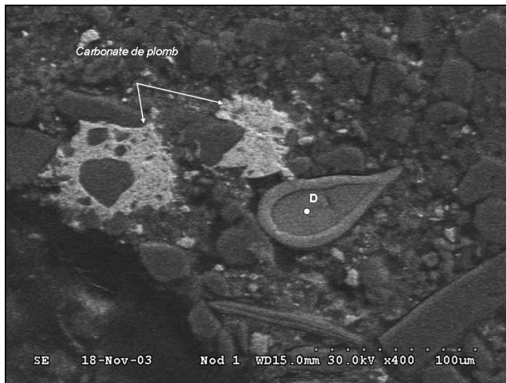
Figure 5 - Secondary electron picture in the dark area of the thin section including the oxidation front.
