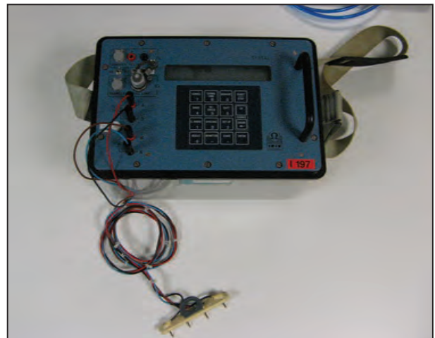
Figure 7 - Resistivity measurement apparatus and cables used for the pedagogic device (Giot G., 2009).
